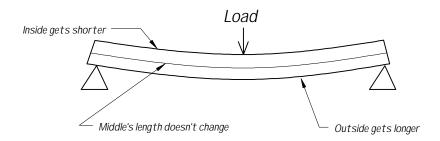
We can remove most of the beam's interior without changing its stiffness very much. The only requirement is that we leave enough interior material so that the outer surfaces cannot collapse toward each other when the beam is bent. A torsion box can achieve almost all of the stiffness of a solid beam even though it is mostly air.
